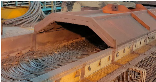
Fig.1. Photo of the Stelmor process and insulation cover.
