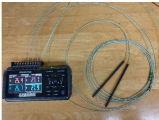
Fig.5. The photo of the rod with an inserted thermocouple.
