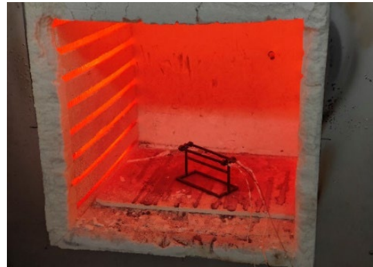
Fig.6. The photo of the support and the rod inside the experimental furnace.
